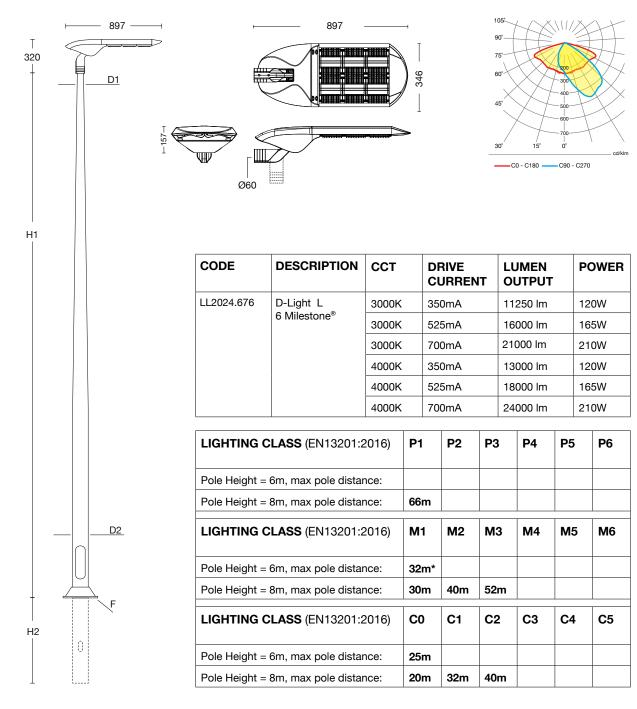
D-Light L 6ML Weight: 14 kg Wind surface area: 0.07 / 0.28 m2
