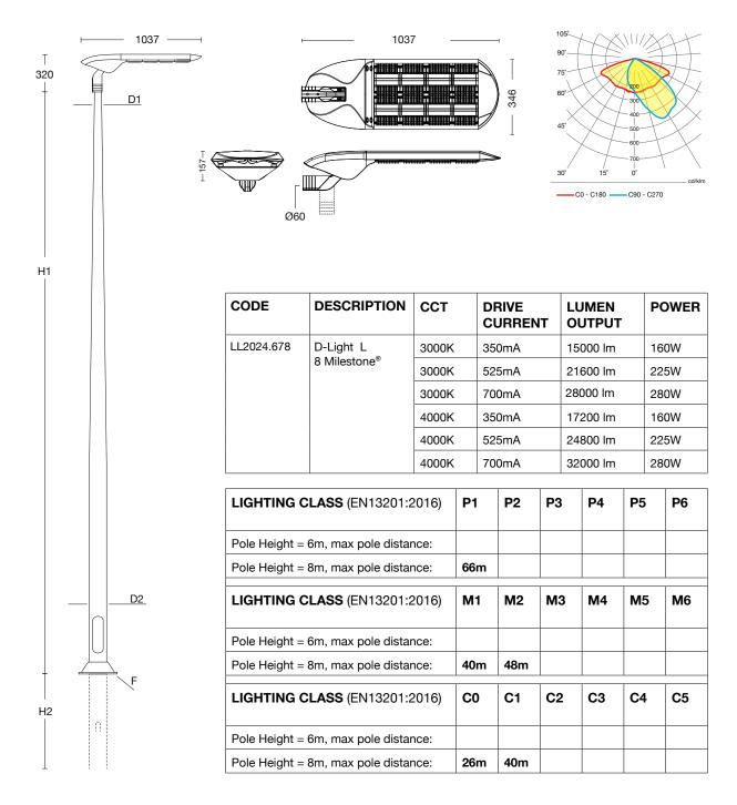
D-Light L 8ML Weight: 11.5 kg Wind surface area: 0.06 / 0.23 m2
