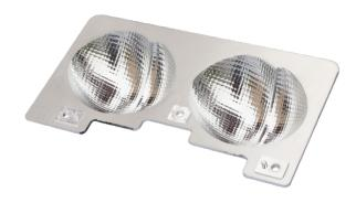
Milestone<sup>®</sup> LED module introduces the indirect lighting concept through its multifaceted reflectors. Light beams coming out of the upward aligned LED chips are reflected in a way that almost sending them horizontally with no uplight. Light can reach spaces that standard lenses can fail to send.
