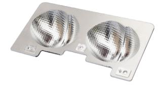
Milestone<sup>®</sup> Evo LED module introduces the indirect lighting concept through its multifaceted reflectors. Light beams coming out of the upward aligned LED chips are reflected in a way that almost sending them horizontally with no uplight. Light can reach spaces that standard lenses can fail to send.
