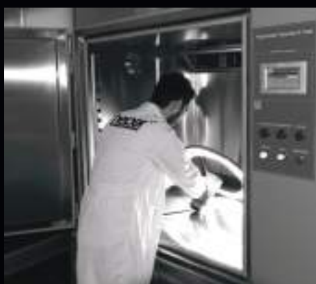
We run tests for various types of materials for their tolerances against heat, cold, aridity and humidity, simulating different world climates.
