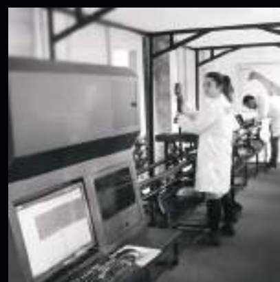
We run photobiological safety tests to see the blue light hazard in our lighting fixtures.
