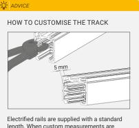
Electrified rails are supplied with a standard length. When custom measurements are needed, they must be cut with a hacksaw or circular saw suitable for aluminum. After cutting the track you must shorten the contacts with the appropriate accessory (1099258X) to a length of at least 5 mm.
