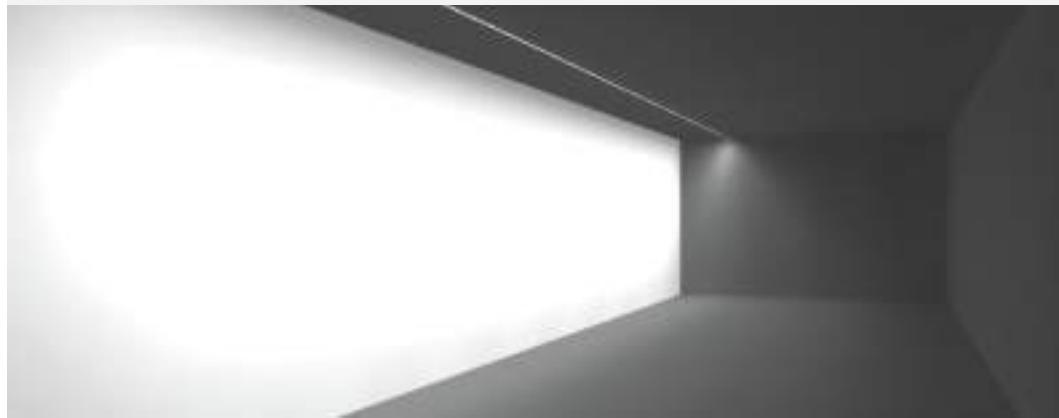
Wall Washer optics provides a uniform illumination of large vertical surfaces. By emphasizing walls, it creates a visual expansion effect to make spaces brighter and higher.
